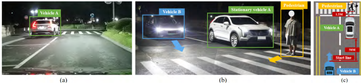
Figure 11: (a) Rear view of Vehicle A . The pedestrian positioned ahead of Vehicle A remains invisible to the direct line of sight from Vehicle B . (b) Side view of the experimental scene. (c) Schematic diagram of the experimental scenario.
