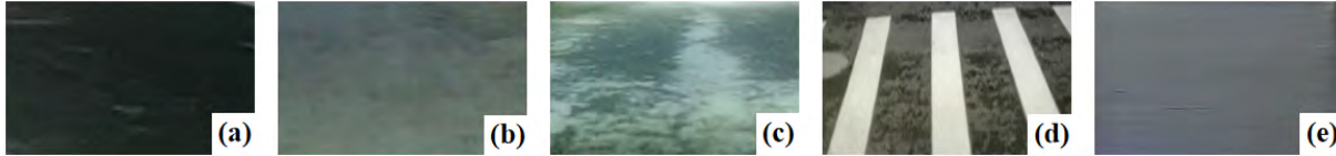
Figure 17: Five types of road surface: (a) wet tarmac road: after rained moderately, (b) dry tarmac road, (c) tarmac road not completely dry: two hours after moderate rain at 30 °C, (d) crosswalk, (e) garage floor with epoxy paint.
