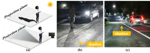
Figure 2: (a) Shadow projection schematic. (b) Shadow casted by pedestrian with a close up view. (c) A rear view of shadow casted by pedestrians.
