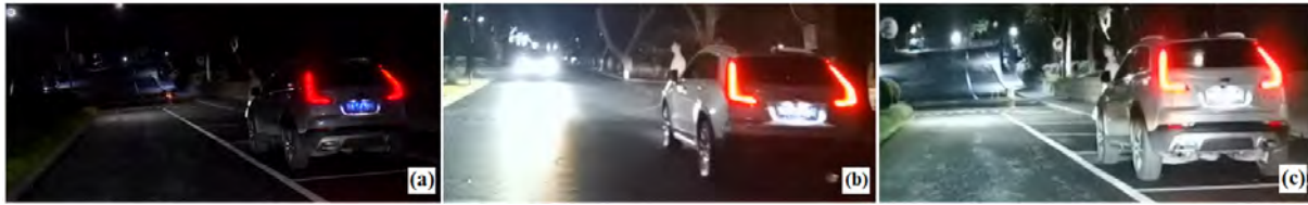
Figure 16: Three types of illumination situation: (a) Dark, (b) Opposite lights, (c) Road lights.
