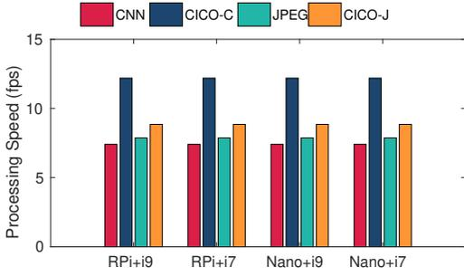
Figure 16: Processing speed using LTE (CLS).
