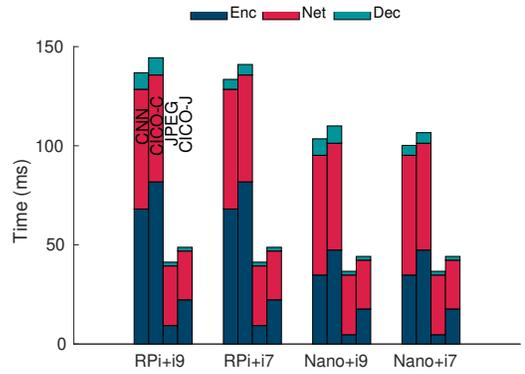
Figure 13: End-to-end offloading latency using WiFi (DET).
