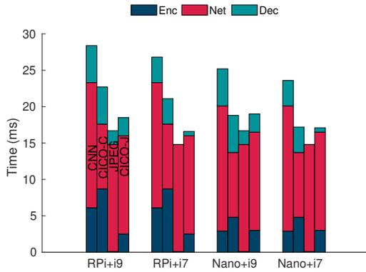
Figure 11: End-to-end offloading latency using WiFi (CLS).
