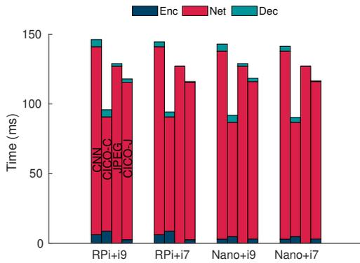
Figure 12: End-to-end offloading latency using LTE (CLS).
