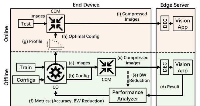
Figure 2: System Architecture
