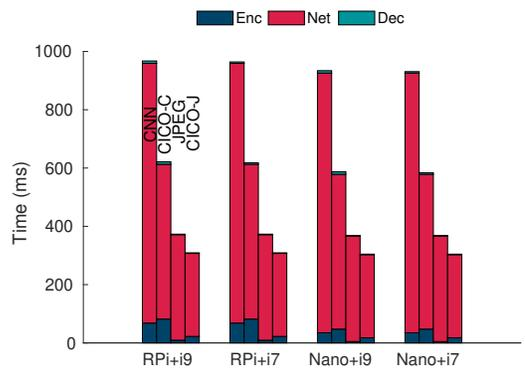
Figure 14: End-to-end offloading latency using LTE (DET).
