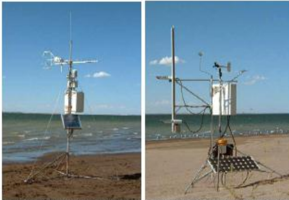
Figure 3. (left) Campbell Sci. CSAT3 3D sonic system, and (right) REBS Bowen ratio system.
