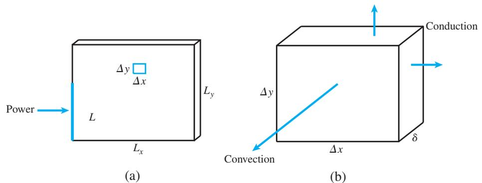
**Figure 8.15 Cooling fin in Reality Check 8.** (a) Power input occurs along interval  $[0, L]$  on left side of fin. (b) Energy transfer in small interior box is by conduction along the  $x$  and  $y$  directions, and by convection along the air interface.
