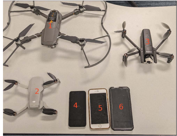
Figure 7: Six devices used in the experiment: a DJI Mavic Zoom drone labeled 1, a DJI Mavic Mini drone labeled 2, a Parrot Anafi Thermal drone labeled 3, and 3 smartphones: an Honor View 10 labeled 4, an iPhone 6s Plus labeled 5, and an HTC One Plus 7 Pro labeled 6
