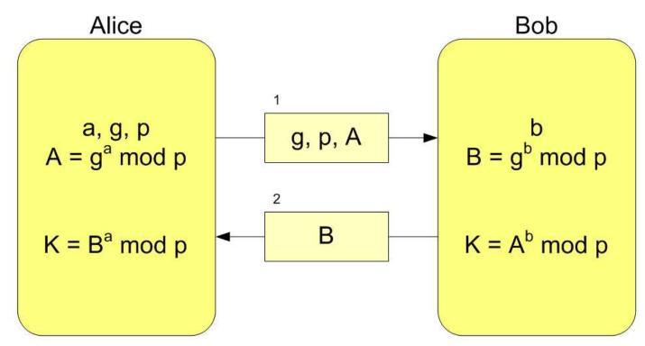
$K = A^b \mod p = (g^a \mod p)^b \mod p = g^{ab} \mod p = (g^b \mod p)^a \mod p = B^a \mod p$
