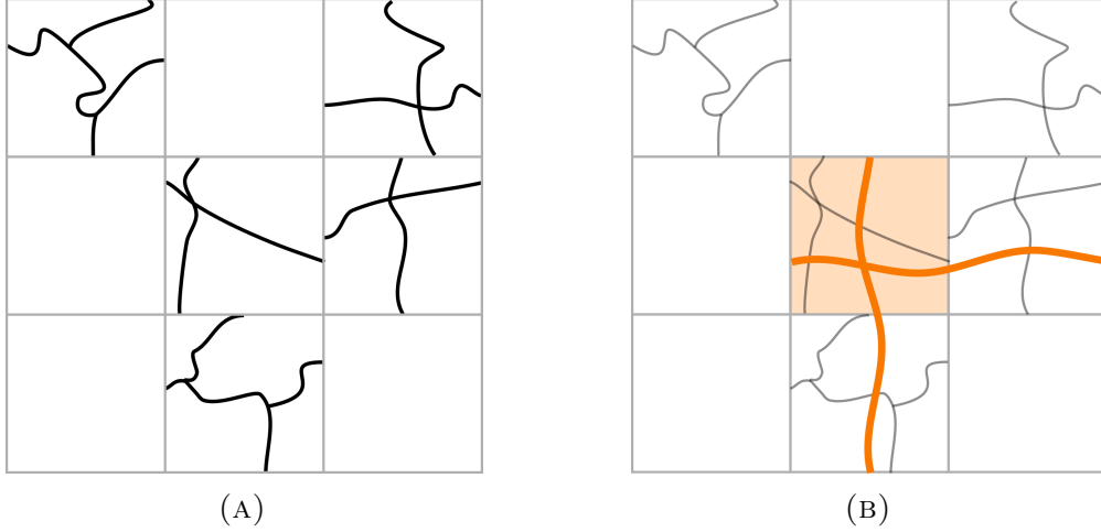
FIGURE 2. (A) A full renormalized site contains a designated set of microscopic bonds which is connected and crosses the site in both horizontal and vertical directions. (B) Such a site is declared open if its designated bond set is connected with that of each of its full neighbors. We construct open sites by finding rectangle crossings in an adjacent slab, and adding “pins” of bonds at overlap points.
