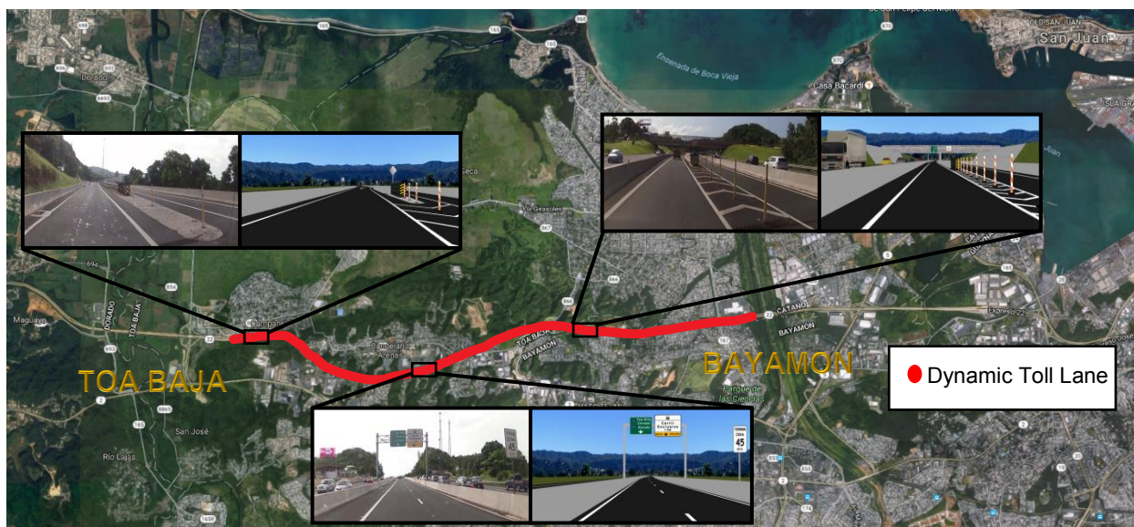
Figure 1.2 Reversible Dynamic Toll Lane System in PR-22
