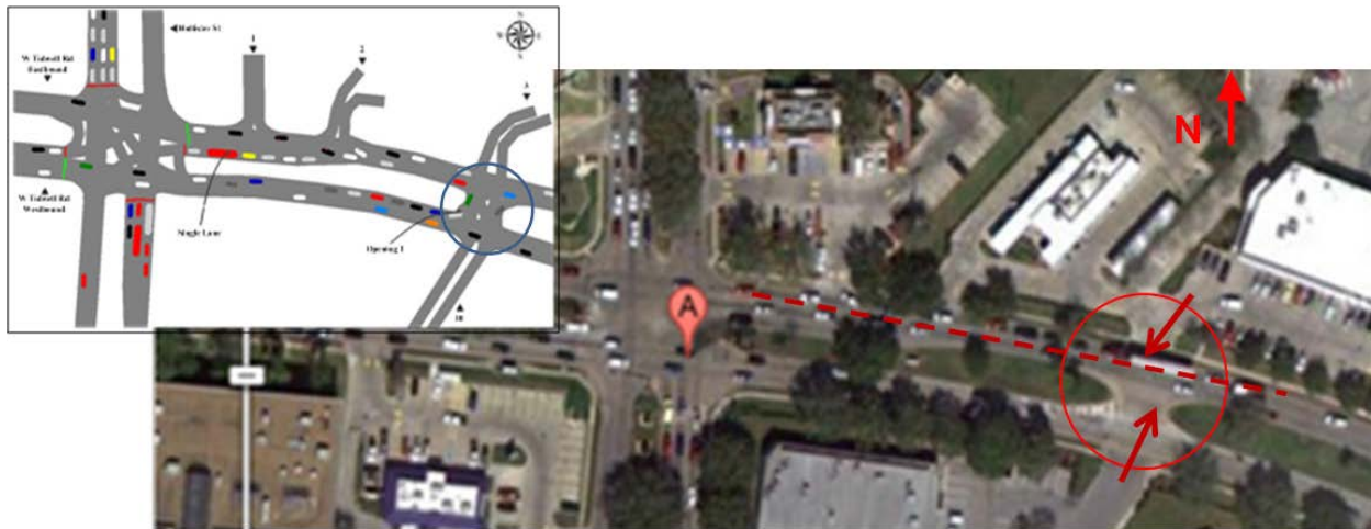
Figure 9-3. Interference between Through Vehicles and Left-Turn Vehicles Egressing from the Driveways in the Base Case.
