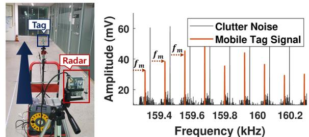
**Figure 8: The spectral leakage in a mobile tag.**
