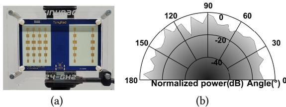
Figure 14: (a) OmniScatter reader implemented on Eval-Tinyrad, and (b) the single Tx antenna omni-directional beam pattern
