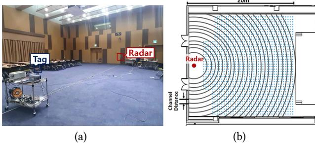
Figure 18: Large-scale evaluation in an auditorium of over  $20\text{m} \times 20\text{m}$ : (a) on-site view and (b) deployment scenario where the blue dots and coaxial circles indicate tags and channels, respectively.
