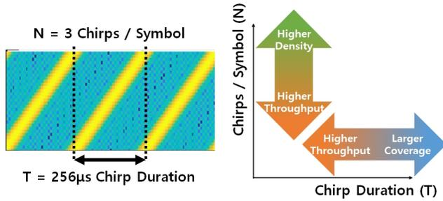
**Figure 6: The coverage of HD-FMCW grows proportional to chirp duration  $T$  and the density grows proportional to the number of chirps  $N - 1$ . The chirp duration and samples per chirp collectively form the per-tag throughput proportional to  $\frac{1}{T \times N}$ .**
