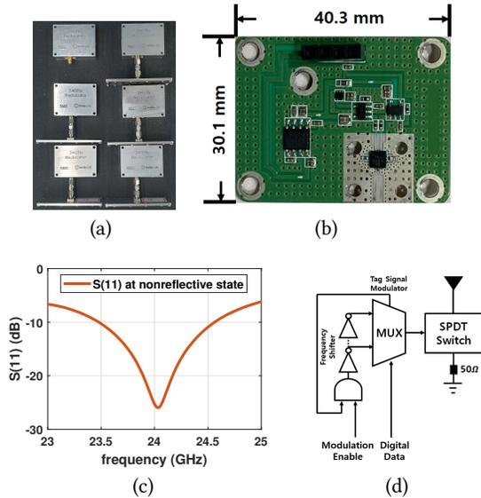
**Figure 9: (a) 6 of our mmWave tags inside the aluminum casing. (b) Our mmWave tag board. (c) The  $S(11)$  parameter of our tag at  $50 \Omega$  matched ground (non-reflective) state. (d) The tag’s circuit diagram.**
