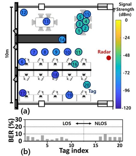
Figure 12: (a) Signal strength and (b) BER of the tag with a single omni-directional radar. Signal strength as low as -103.6 dBm achieves < 10% BER
