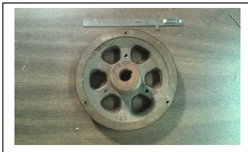
The treadmill's flywheel, drilled and tapped for blade attachment
