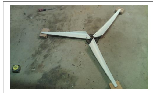
To ensure the blades were attached symmetrically, I used a tape measure to get the tip-to-tip spacing precise before drilling the final attachment holes through the blade.
