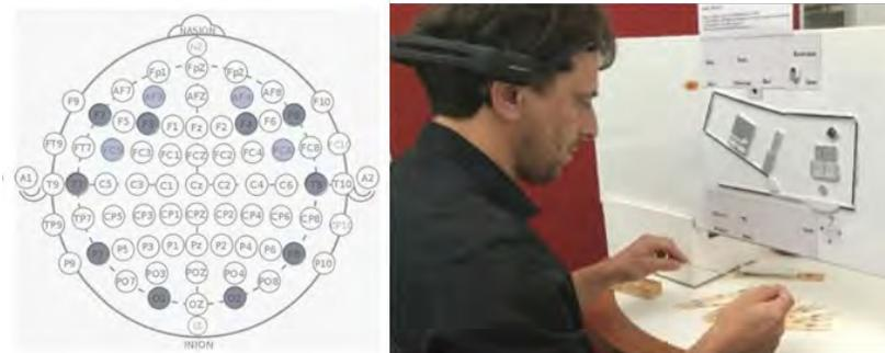
Figure 2. Emotiv Epoc+ electrodes arrangement (10-20 I.S.) and experiment setup using the headset.
