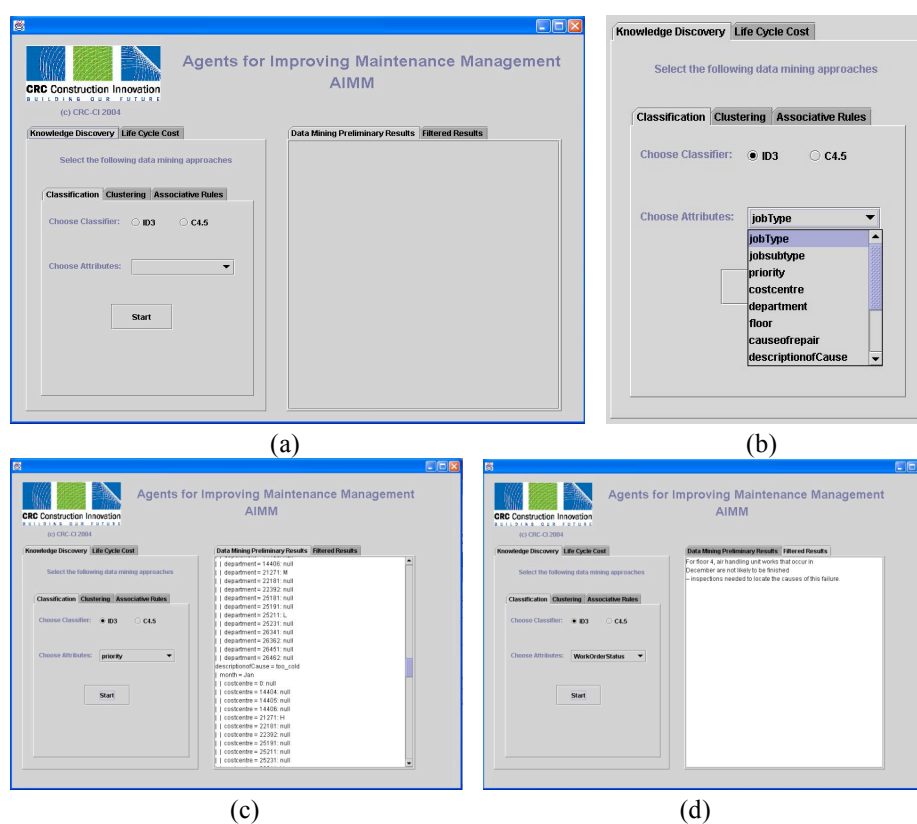
Figure 4. (a) The AIMM prototype system is instantiated once a building asset type has been selected; (b) Data mining techniques and different attributes for the user to choose from based on focus and interest; (c) Preliminary results of applying the ID3 with the “Priority” attribute on the maintenance data of Air Handling Unit; and (d) An example of the filtered knowledge presented to the user from the preliminary results of applying the ID3 with the “Work Order Status” attribute on the maintenance data of Air Handling Unit.
