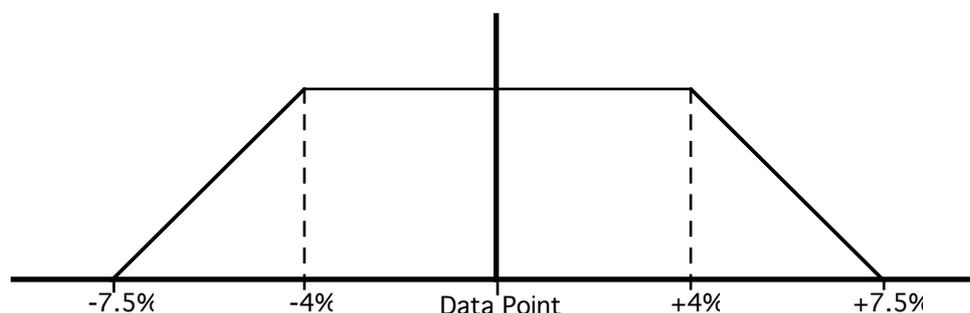
Fig. 7. Trapezoidal filter used for the moving weighted average.
