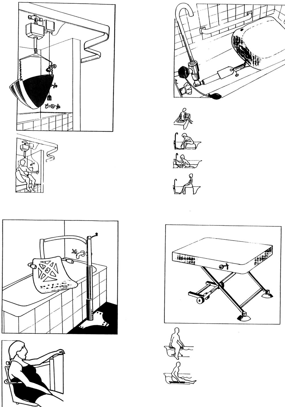
Figure 3 Illustrations of four devices designed to assist the elderly in entering and leaving a bath.
