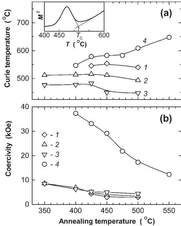
**Figure 6.** Effect of annealing temperature on (a) Curie temperature and (b) room-temperature coercivity for (1)  $\text{SmCo}_4\text{Cu}_1$ , (2)  $\text{SmCo}_{3.5}\text{Cu}_{1.5}$ , (3)  $\text{SmCo}_3\text{Cu}_2$  and (4)  $\text{SmCo}_{2.25}\text{Fe}_{0.75}\text{Cu}_2$ . The inset shows an example of  $T_C$  evaluation ( $\text{SmCo}_{3.5}\text{Cu}_{1.5}$ ,  $T_A = 400^\circ\text{C}$ ).
