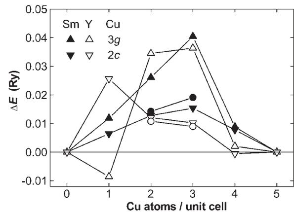
**Figure 2.** Deviation of the  $\text{RCo}_{5-x}\text{Cu}_x$  energy from that for the  $\text{RCO}_5 + \text{RCu}_5$  mixture calculated by LAPW for magnetic  $\text{SmCo}_{5-x}\text{Cu}_x$  ( $\bullet, \blacktriangle, \blacktriangledown$ ) and non-magnetic  $\text{YCo}_{5-x}\text{Cu}_x$  ( $\circ, \triangle, \nabla$ ) with the  $\text{Cu}$  atoms preferring  $3g$  sites,  $2c$  sites ( $\blacktriangle, \triangle$ ), or having no preferential site occupancies ( $\bullet, \circ$ ).
