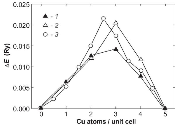
**Figure 1.** Deviation of the  $\text{RCo}_{5-x}\text{Cu}_x$  energy from that for the  $\text{RCO}_5 + \text{RCu}_5$  mixture calculated (1) by LAPW for  $R = \text{Sm}$ , (2) by LAPW for  $R = \text{Y}$  and (3) by LMTO-ASA for  $R = \text{Y}$ . All the compounds are magnetic and the  $\text{Cu}$  atoms prefer the  $2c$  sites.
