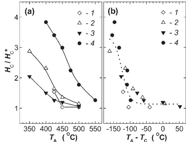
**Figure 7.** Reduced coercivities of (1)  $\text{SmCo}_4\text{Cu}_1$ , (2)  $\text{SmCo}_{3.5}\text{Cu}_{1.5}$ , (3)  $\text{SmCo}_3\text{Cu}_2$  and (4)  $\text{SmCo}_{2.25}\text{Fe}_{0.75}\text{Cu}_2$  after annealing versus (a) annealing temperature  $T_A$  and (b) deviation of  $T_A$  from the Curie temperature  $T_C$ .  $H_c^*$  is the coercivity before annealing.
