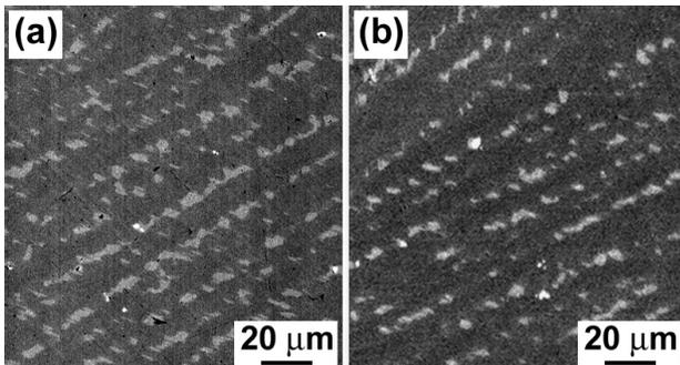
**Figure 4.** SEM backscattered electron images of  $\text{SmCo}_3\text{Cu}_2$  samples: (a) the as-made alloy and (b) alloy annealed at  $350^\circ\text{C}$  have a two-phase structure.
