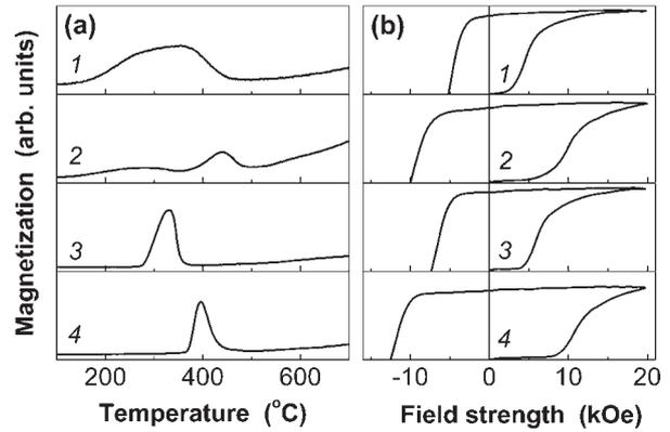
**Figure 5.** (a) Thermomagnetic curves and (b) magnetization curves of the  $\text{SmCo}_3\text{Cu}_2$  alloy: as-made (1); annealed at  $350^\circ\text{C}$  (2); homogenized at  $1050^\circ\text{C}$  (3); homogenized at  $1050^\circ\text{C}$  and annealed at  $350^\circ\text{C}$  for 200 h (4).
