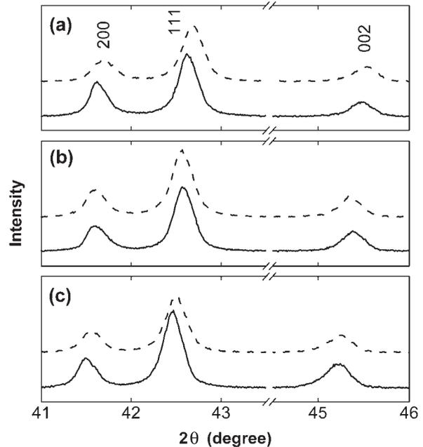
**Figure 8.** Experimental XRD spectra for (a)  $\text{SmCo}_4\text{Cu}_1$ , (b)  $\text{SmCo}_{3.5}\text{Cu}_{1.5}$  and (c)  $\text{SmCo}_3\text{Cu}_2$ , annealed at  $350^\circ\text{C}$  (—) and at  $500^\circ\text{C}$  (---).
