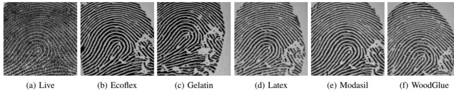
Fig. 2. Materials used to fabricate the spoof samples taken from LivDet 2013 databases.
