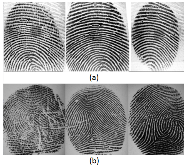
Fig. 18. Examples of live (a) and spoof (b) fingerprint images from the dataset assembled by the organizers of the LivDet competition. Spoof are realized using latex, gelatin and ecoflex, respectively. With permission of G. Marcialis.
