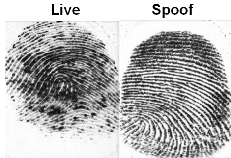
Fig. 15. Grey-level uniformity analysis in real and spoof fingerprint images. Images taken from the LivDet 2009 database, with permission of G. Marcialis.
