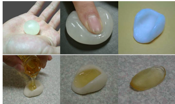
Fig. 6. Making an artificial fingerprint directly from a live finger: plastic is used to obtain the mold and gelatin to obtain the cast. Image taken from [ http://web.mit.edu/6.857/OldStuff/Fall03/ref/gummy-slides.pdf ], with permission of Dr. T. Matsumoto.
