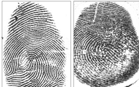
Fig. 24. Spoof fingerprints obtained using the same material (silicone) but scanned by two different optical devices (CrossMatch and Biometrika respectively) taken from LivDet09, with permission of G. Marcialis.
