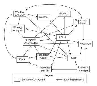
Figure 1: Subset of EDS Software Architecture
