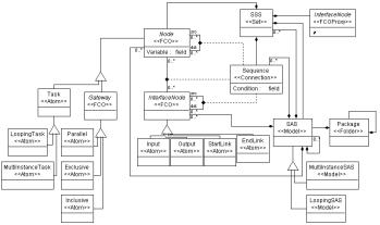
Figure 3. Subset of the SAS meta-model in GME.
