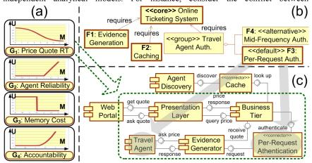
**Fig. 1.** Travel Reservation System: (a) goals, (b) features, thick border indicates a feature that is enabled, (c) software architecture corresponding to the enabled features.
