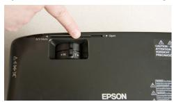
8. Adjust height of display on Projection Screen by pressing button to raise or lower Projector Foot.
